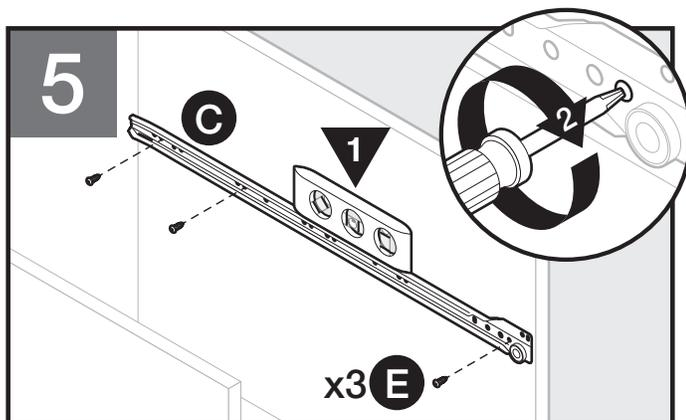
Make sure cabinet member (C) is level; secure with screws (E). Repeat Steps 4-5 for remaining cabinet member (A).
