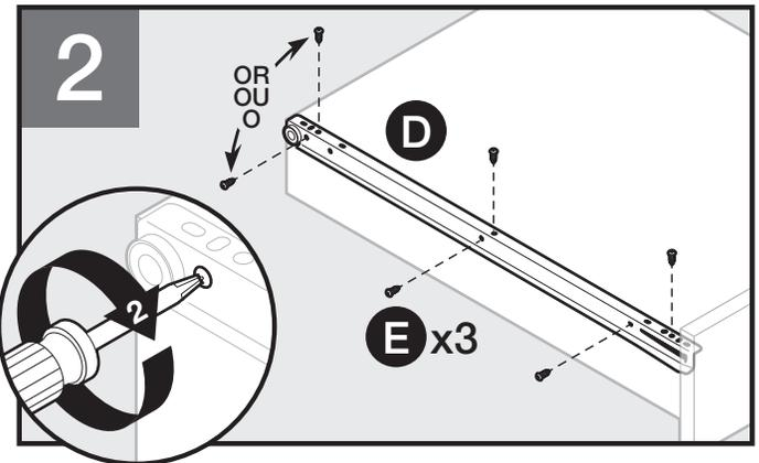
Secure with screws (E). **NOTE:** Drawer member can be secured on top or sides. Repeat Steps 1-2 for remaining drawer member (B).
