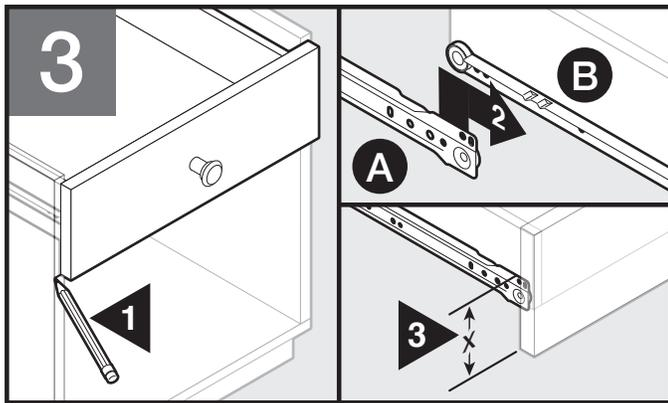
Determine drawer position. Mark bottom of drawer front. Place cabinet member (A) onto drawer member (B). Measure "X".
