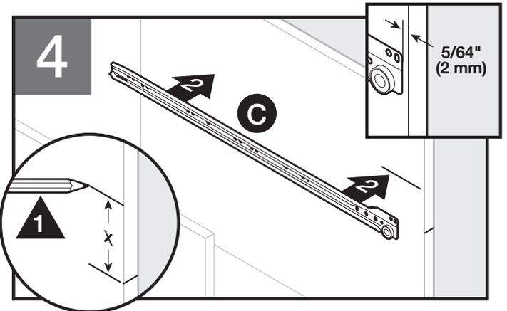
Mark "X" from bottom of mark. Align top of cabinet member (C) with mark, 5/64" (2 mm) from front of cabinet.
