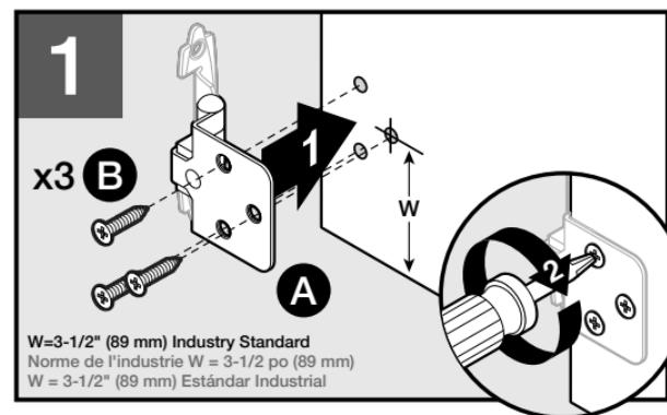
Attach hinges (A) to door with screws (B).
