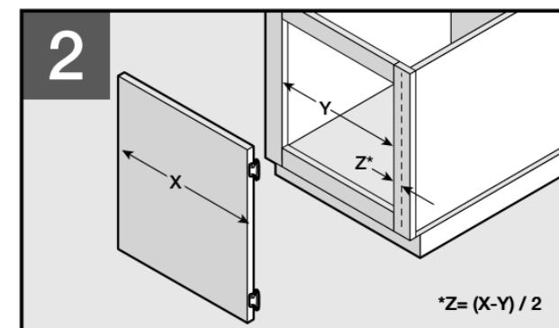
To determine correct overlay, subtract cabinet opening "Y" from door width "X" and divide by 2. Mark "Z" on face-frame with a piece of tape.
