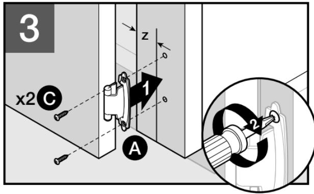
Line up edge of cabinet door with "Z" mark. Adjust door vertically as needed. Secure with screws (C). Remove tape from face-frame.
